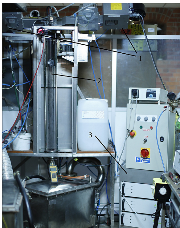
Figure 2. The microwave plasma reactor: 1 – microwave generators, 2 – quartz tube, 3 – power supply
